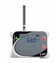
GSM datalogger is designed to record  $\mathrm{CO}_2$  from built-in sensor. In case of exceeded set limits, SMS and JSON messages can be sent via GPRS data connection. It is possible to set the regular sending of JSON messages to COMET Database, the sending interval is adjustable. Alarms are also indicated locally by LED, LCD and acoustically by built-in beeper. The recording is performed in a non-volatile electronic memory. The data can be transferred to a PC via USB-C.
